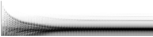
Figure 2. Sine map. F = 880 hz, C = 4 , window length 0.2 seconds. It takes about one minute for the vibrato to decay to an imperceptible level. This constant Q filterbank analysis with semitone spacing of analysis bands shows the first 20 seconds.
